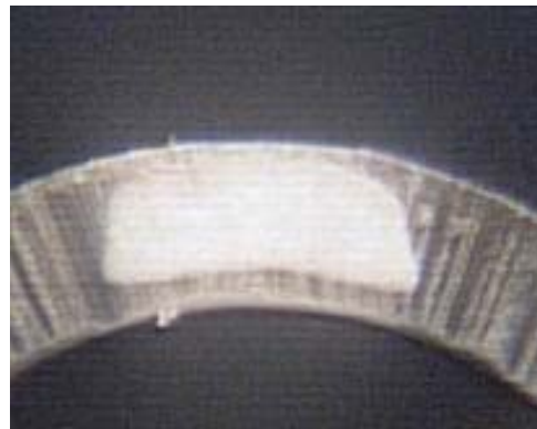
Figure 5. Interface shape of the coextrusion sample at the same temperature of 210°C for both TPU and filled TPU.
